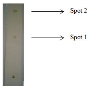
Figure 2. Test for the presence of Lutein by TLC
